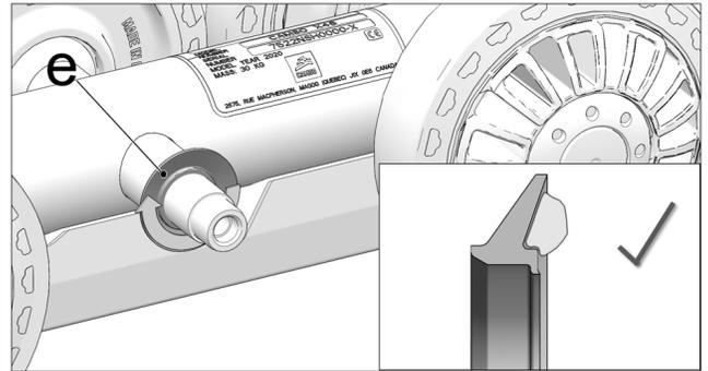
2.2 Apply evenly 3 to 3.5 cc of grease in v-shaped groove (e), all the way around.
