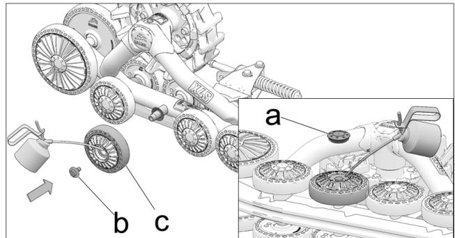
2.4 Slide new wheel (c) on shaft, making contact with seal. Install new bolt (b) and tighten to **30 N-m** (22 lb-ft) of torque.
