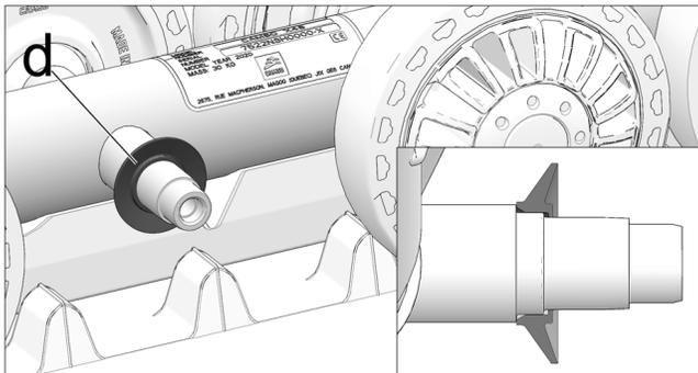
2.1 Install new seal (d) on clean, dry wheel shaft at position shown above.
