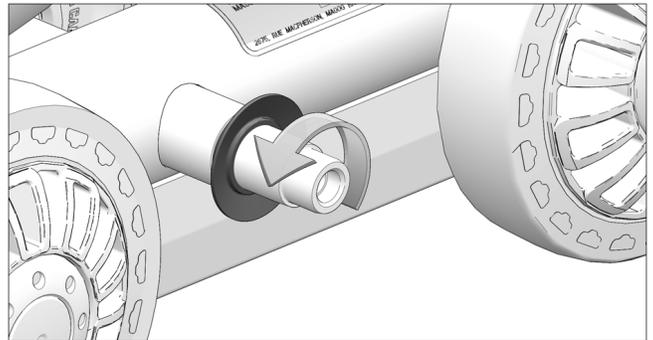
2.3 Apply grease evenly on shaft where new wheel will be mounted.
