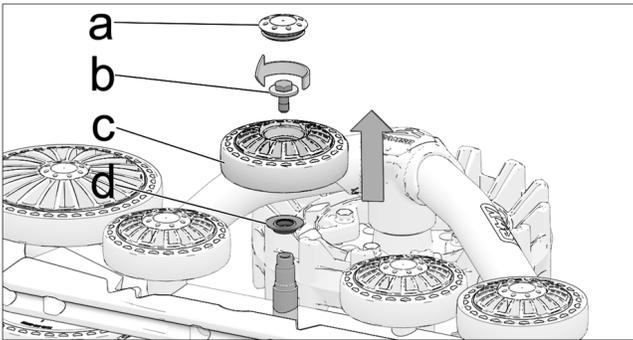
1.1 Remove cap (a), loosen and remove bolt (b), lift wheel (c) off of wheel shaft, remove wheel seal (d).
