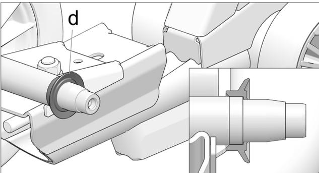
2.1 Install new seal (d) on clean, dry wheel shaft at position shown above.
