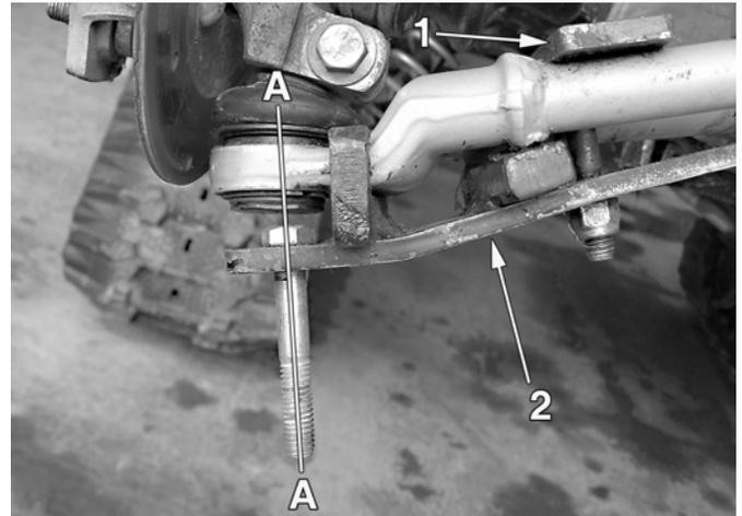
6. Using the nuts (18) provided, secure undercarriages to front wheel hubs. The procedure and precautions are the same as for rear units. Refer to Figure 13 for reference.
