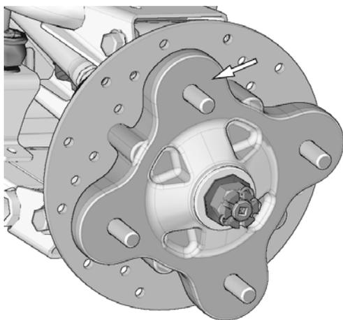
3. If applicable, remove CV joint protectors.
