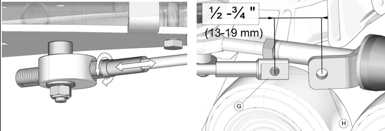
16. Reverse steering wheel a little to be able to bolt support plate and cable together. Tighten provided bolt (**i**) to 35 N•m [24 lb•ft]. See Figure 28. Repeat steps for right side.
